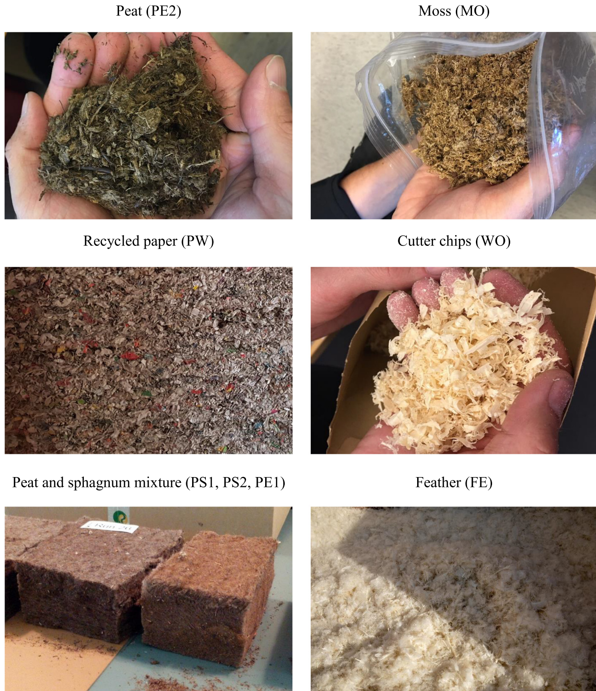
Fig. 1. Raw bio-based materials of investigated insulators.
